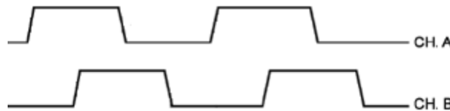
Fig. 4.32: The signals at CH A and CH B outputs of quadrature encoder
